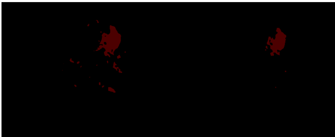
Figure 4-7: Binary image before and after the morphologic opening
